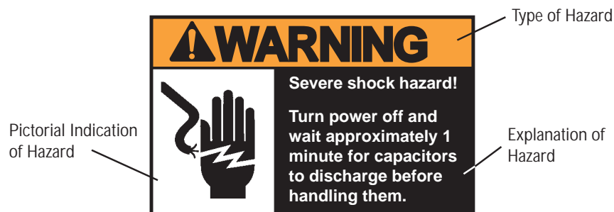
Sample Hazard Alert
