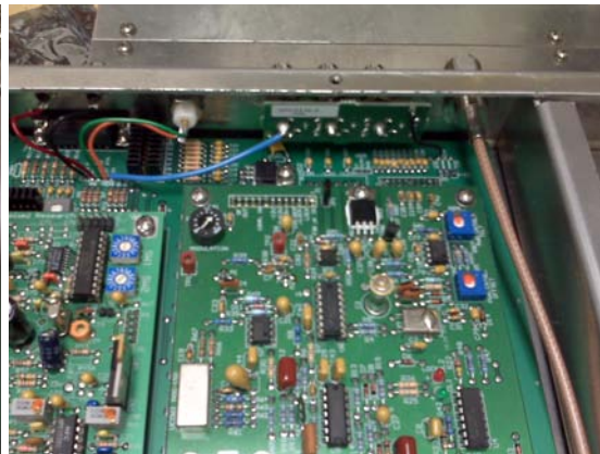
Blue wire moved to BNC connector
