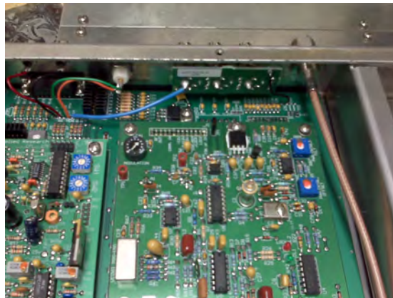
Blue wire moved to BNC connector
