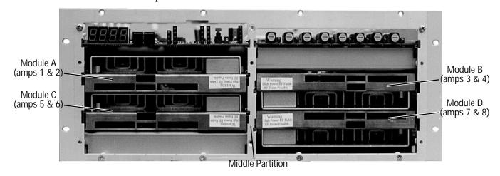
Illustration 2-2 Power Amplifier Module Placement
