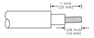
Illustration 2-3 Cover, Cable & Conductors
